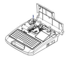
3) Insert the new cutter receiving plate.
