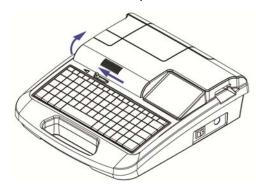
2) Press at the positions shown with arrows and pull the ribbon cassette upward to take it out;
