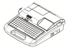
Insert the lock tongue of tube holder in the corresponding slot of printer, and then press down the other end of the tube holder until you hear a clicking sound;
