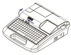
2) Press down the left lock tongue of tube holder and pull the tuber holder upward to take it out as shown in the figure;
