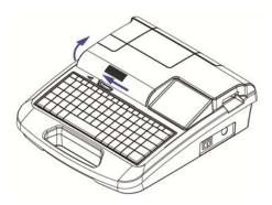
2) Press down the left lock tongue of label cassette and pull the label cassette upward to take it out;
